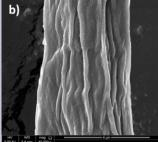
**Figure 2:** a) Representative scanning electron microscope image of the raw and b) alkali-treated *P. undulata* fibers, showing the loss of hemicellulose, lignin, and bioactive extractives from the raw fibers after alkali treatment.
