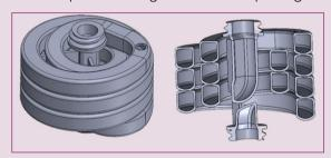
**Figure 3:** The final design of the cartridge with a section view showing the internal details.
