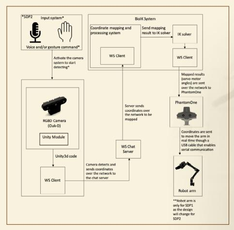
**Figure 1:** High-level architecture of Waleef system.
